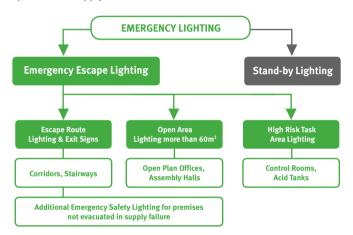
Escape route emergency lighting may be for a corridor, or for delineated routes such as pedestrian routes in a covered car park. Where there is no marked or delineated route open area lighting should be used.
