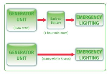
Where generator systems are used for emergency lighting a back up battery will also be required to cover the time taken for the generator to start and run to full power.
